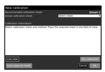
Depending on current zoom level and close-up lens, the app will recommend a calibration sheet for the calibration. Place the recommended calibration sheet straight under your microscope, so that the top row of dots is visible. Here is the list of the range covered by each TAGARNO calibration sheet.
